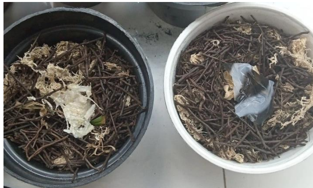
Figure 7. Comparative test of bioplastic degradation with conventional plastic using the method of decomposing soil organisms (before planting in the ground).
