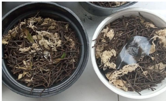
Figure 8. Comparative test results of bioplastic degradation with conventional plastic using the method of decomposing soil organisms after 2 days.
