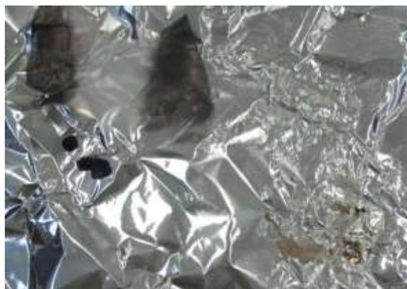
Figure 6. Burning test on conventional plastic (A) and bioplastic (B).
