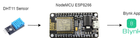
Figure 6. Temperature Monitoring System Design
